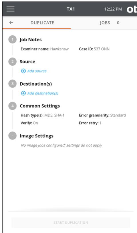
The job setup screen is organized in a natural workflow from top to bottom, but most steps and settings can be accessed in any order. The default values display for each step and setting. Tap on the step number or heading to expand the section and view or change the settings.
