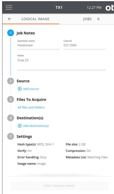
4. To select a filesystem from an available source drive, tap the 2 or Source heading. A list of attached drives will appear, with a filesystem summary tile shown under each drive for any filesystems recognized by TX1. Note that network shares can also be used as logical image job sources. To make a network
