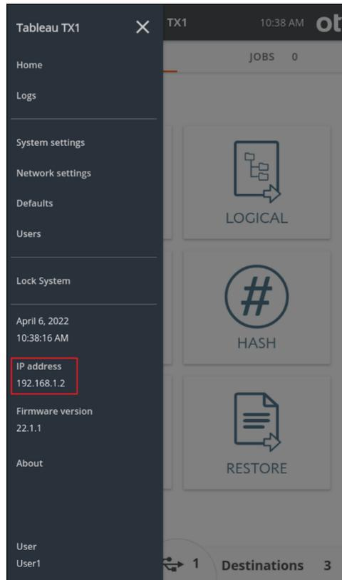
4. Open a web browser of your choice on a computer/device that is connected to the same local area network as TX1, type TX1's IP address (or hostname) into the address field in the web browser (same field where you would enter a web page URL), and press Enter. The remote UI login screen should be shown in your browser.
