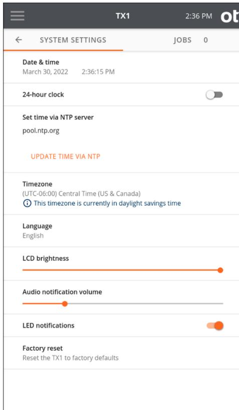
The **System Settings** page provides selections to configure basic TX1 system options including **Date & time**, **24-hour clock**, **Set time via NTP server**, **Timezone**, **Language**, **LCD brightness**, **Audio notification volume**, and **LED notifications**. You can also perform a factory reset.
