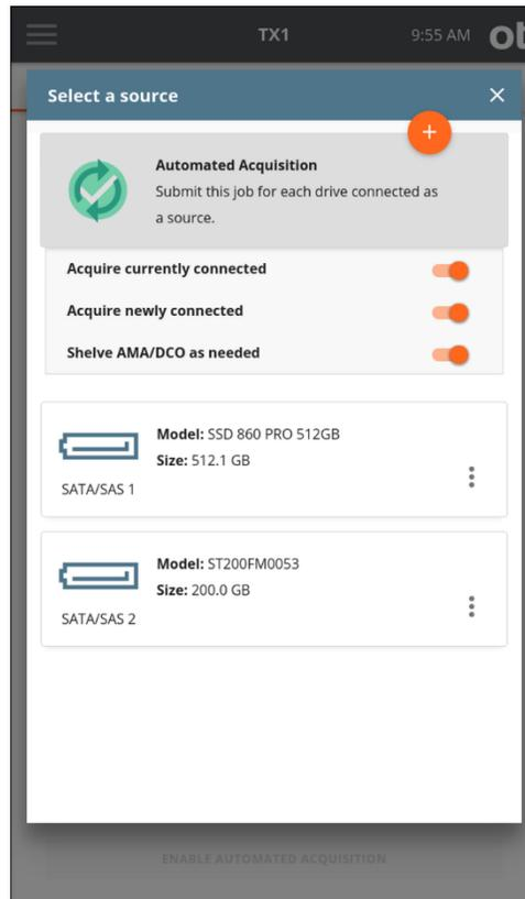
4. Your selection of Automated Acquisition mode will be confirmed by the automated acquisition icon in the left side of the drive tile turning green with a gray checkmark inside. Close the modal by tapping the **X** in the upper right corner or by tapping outside of the modal.
