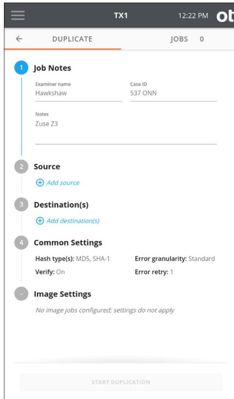
3. To set TX1 into Automated Acquisition mode, tap the **2** or **Source** heading. The top source drive tile is used for automated acquisition setup and will be present whether other source drives are connected or not. Tap the **Automated Acquisition** setup tile to start the automated job configuration process. Three options will be shown that need to be set before proceeding, as follows (and as shown in the screenshot below):
