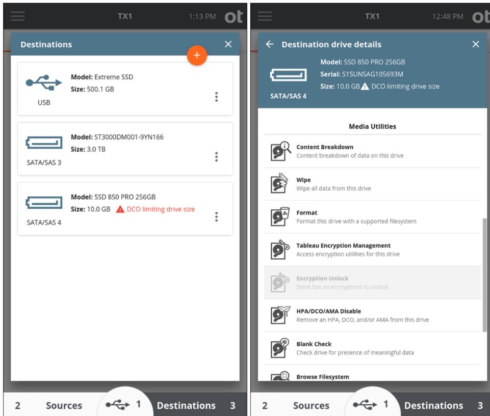
IDE drives with a DCO require special considerations with TX1. This is due to the fact that IDE drives are connected via the PCIe interface using a Tableau IDE Adapter (TDA7-5). DCO setting changes require power-cycling the drive which, for directly connected SATA drives, is done automatically by TX1. PCIe, as implemented on TX1, does not allow for hot drive removal (including power-cycling).
