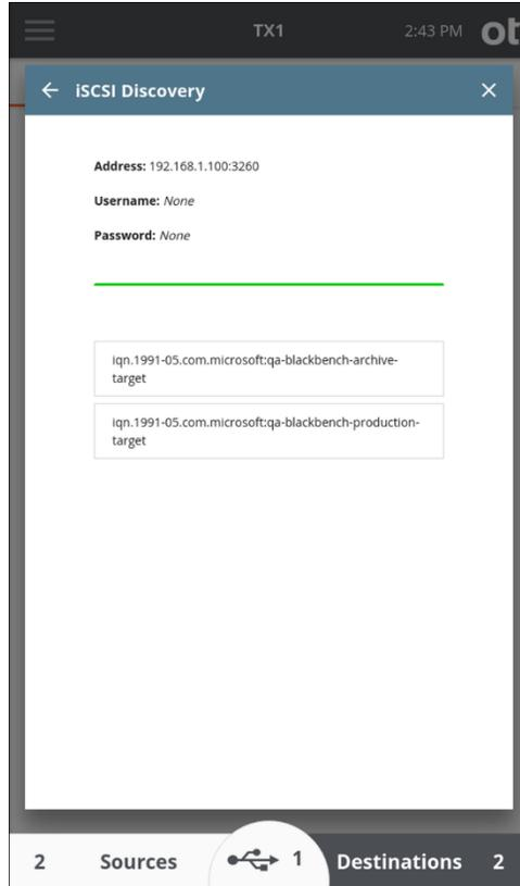
4. Tap an iSCSI target and the **iSCSI Login** screen is displayed. If needed, enter a login username, password, and a nickname (optional). Tap the **Login** button to login and mount the iSCSI target.
