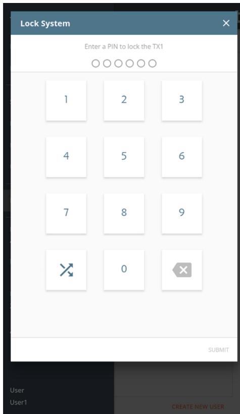
After entering the desired PIN, tap the **Submit** button in the lower right corner of the screen to begin the locking process. The system will prompt you for a second entry of the same PIN to confirm the desired digits have been entered. After verifying that both PINs match, the system will be locked. A message will appear at the top of the lock screen stating the time at which the system was locked.
