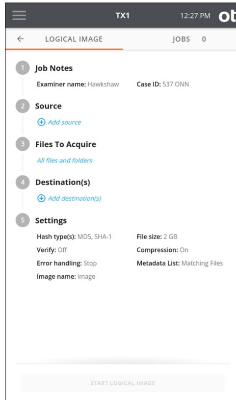
The job setup screen is organized in a natural workflow from top to bottom, but the steps and settings can be accessed in any order. The default values display for each step and setting. Tap the step number or heading to expand the section and view or change the settings.
