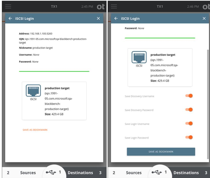
6. The target should now be listed in the Sources or Destinations drive list, depending on where you chose to mount it. The target can now be accessed like a normal drive for Duplication as a source (if mounted as a source), Duplication as a destination (if mounted as a destination), Hash (as a source), Verify (as a destination), and some media utilities.
