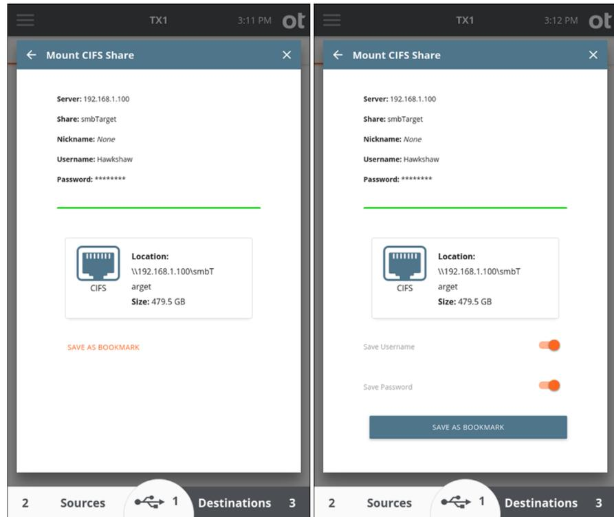
7. The bookmark is now saved (if selected). The share can now be accessed like any mounted filesystem for logical acquisition as a source (if mounted as a source), as a destination for physical and logical image files (if mounted as a destination), Verify (as a destination), Restore (as a source or destination), and some media utilities.
