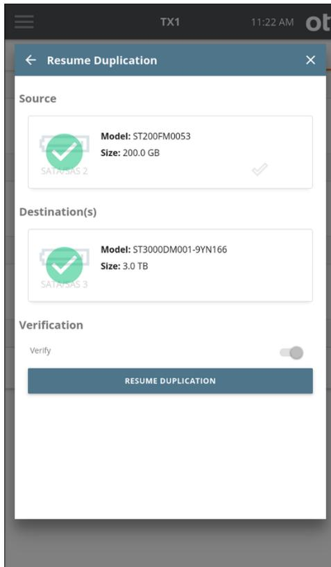
In addition to manually initiated pause and resume, TX1 supports power loss situations as well. For the supported job types (e01, ex01, dd, dmg), if power is unexpectedly lost during an imaging job, it can be resumed after power is restored and the system is booted up.
