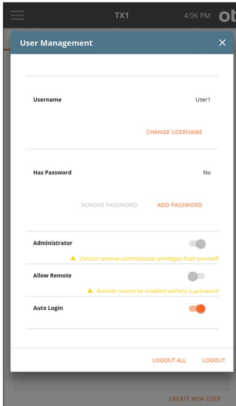
On this screen, an administrator can change any user's username and password, as well as set administrator rights, allow remote access, and enable auto login. Note that remote access cannot be enabled for any users that have no password setup, and auto login cannot be enabled for any that do have a password setup. Also, turning off administrator rights for a currently logged-in administrator is disallowed.
