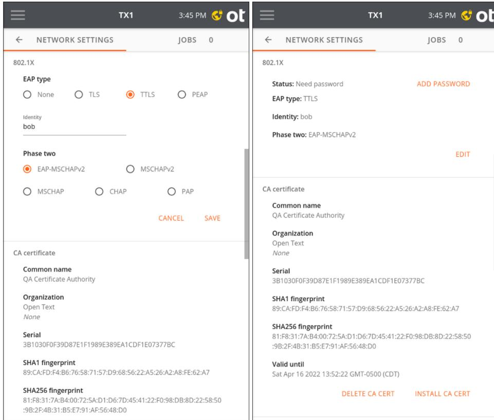
**PEAP:** Select a supported **Phase two** internal protocol (**EAP-MSCHAPv2** or **MSCHAPv2**). A CA certificate must be installed on TX1 to enable server authentication. This method uses an identity and password for client authentication. A client certificate is not required.
