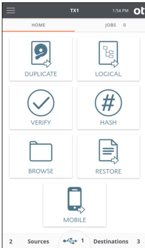
Tap one of these icons to begin a job and enter the job setup screen. A job setup screen provides a stepper-based flow from which you can view default settings,
