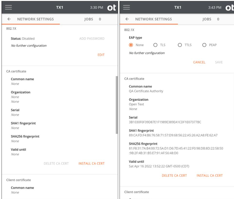
Then tap **Identity** to enter your 802.1X identity (required). Note that each EAP type has additional requirements and configuration settings depending on the type selected, as covered in the sections below.
