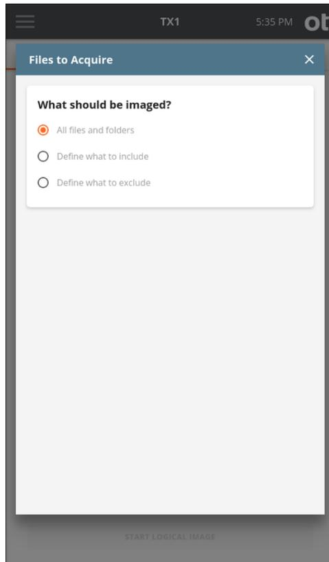
As shown in the screenshot above, the default setting of **All files and folders** is initially selected. If no source file or folder down-selection is desired, simply exit this step by closing the **Files to Acquire** modal window by tapping the X in the upper right corner or by tapping outside of the modal.
