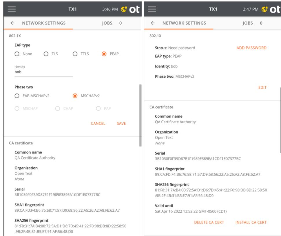
After saving the selected EAP type and **Phase two** internal protocol settings, a yellow icon appears in the right side of the top navigation bar, and an **Add Password** button becomes active in the settings summary area. Tap the navigation bar icon or Add Password to enter an 802.1X passphrase/password. Tap Submit to begin the authentication procedure.
