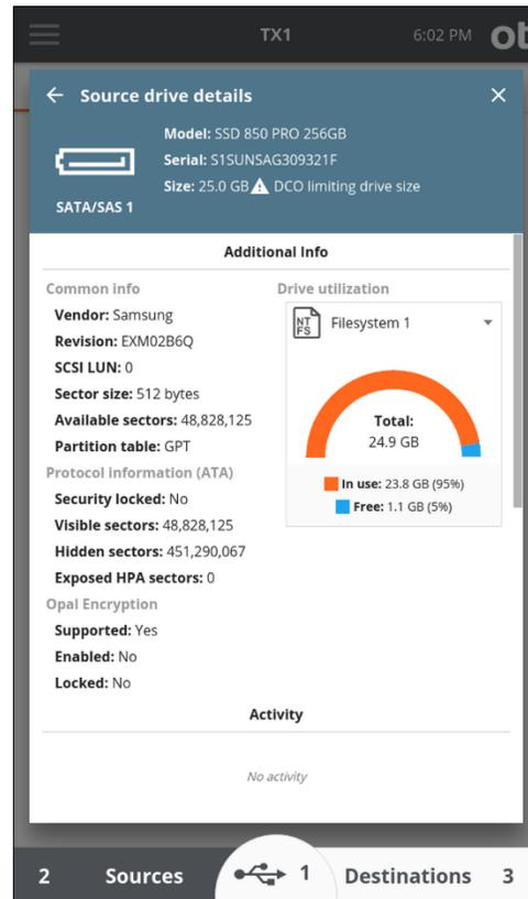
Select a filesystem to display **In use** and **Free** utilization information. Note that changing this selection from Entire drive to one of the detected filesystems only changes the utilization information displayed in this specific sub-area of this screen. All other information on this screen reflects the entire drive, and the media utilities below will act on the entire drive.
