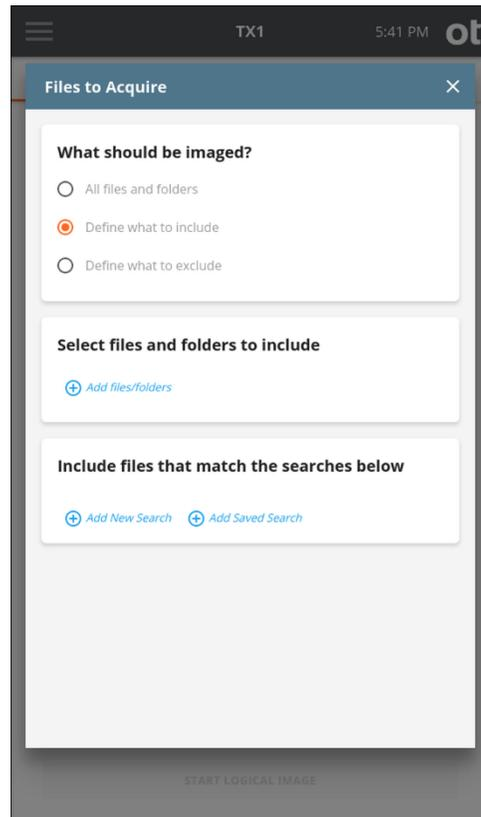
In the example shown above, **Define what to include** is selected, which means the initial acquisition dataset is empty. To manually select which files and folders to include, tap the blue circle/plus sign icon labeled **Add files/folders** in the **Select files and folders to include** section. This will launch a browse modal window which shows the entire contents of the selected source filesystem, as shown below.
