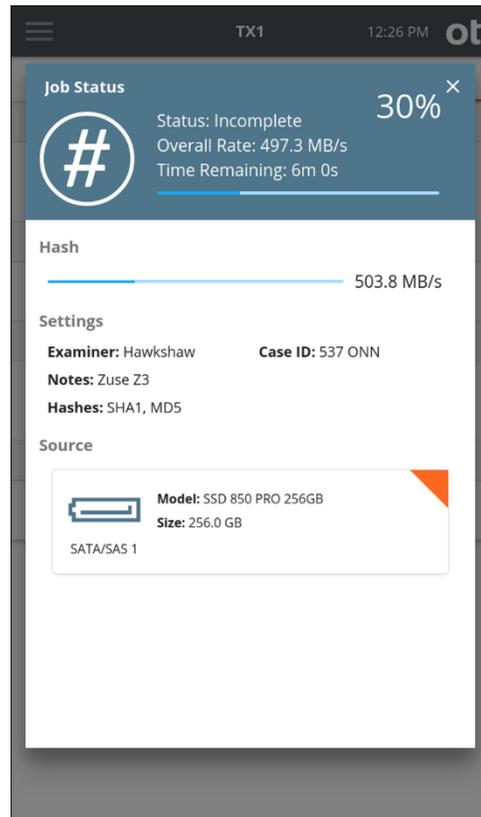
When the hash operation is finished, the results display on the screen. To access the forensic log of the hash job, simply tap the **View Log** button in the header of the completed **Job Status** screen. You can also view the log information by selecting **Logs** from the side navigation menu.
