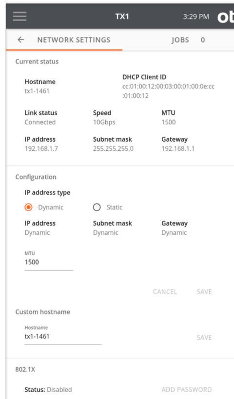
The **Network Settings** screen displays network related information and the current connection status in the top area, followed by a **Configuration** area for setting the IP address, MTU (maximum transmission unit) value, and custom hostname. Following the network configuration area are areas for 802.1X configuration, and an HTTPS certificate area.
