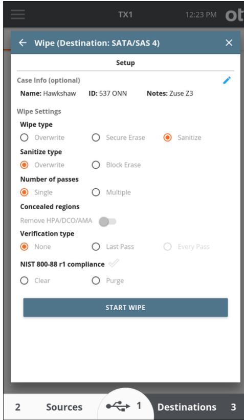
**Note:** Wiping drives results in sustained writing of the media, which can create abnormally high thermal operating conditions inside the drive. OpenText highly recommends using the TX1-S1 drive bay (which has active cooling) or an external drive cooler or fan when wiping media on TX1 to help prevent thermal damage to drives.
