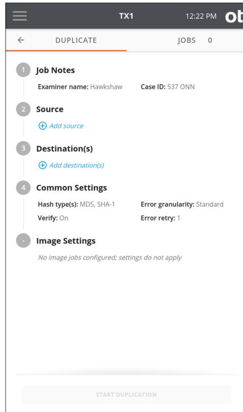
2. To modify or enter job notes, tap the **1** or **Job Notes** heading to expand the section. Tap a text box to modify or enter **Name**, **Case ID**, or **Notes** values and the virtual keyboard is displayed on the bottom half of the screen. If desired, you can also attach a USB keyboard to one of the front Accessory USB ports to make data entry easier. Note that all information entered in the **Job Notes** section will be used for each of the ensuing automated jobs.
