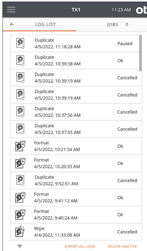
3. Find the desired paused job log (**Paused** status on the right, with the appropriate job start date and time shown) and tap on that log list entry to display the **Log Details** screen for that job log.
