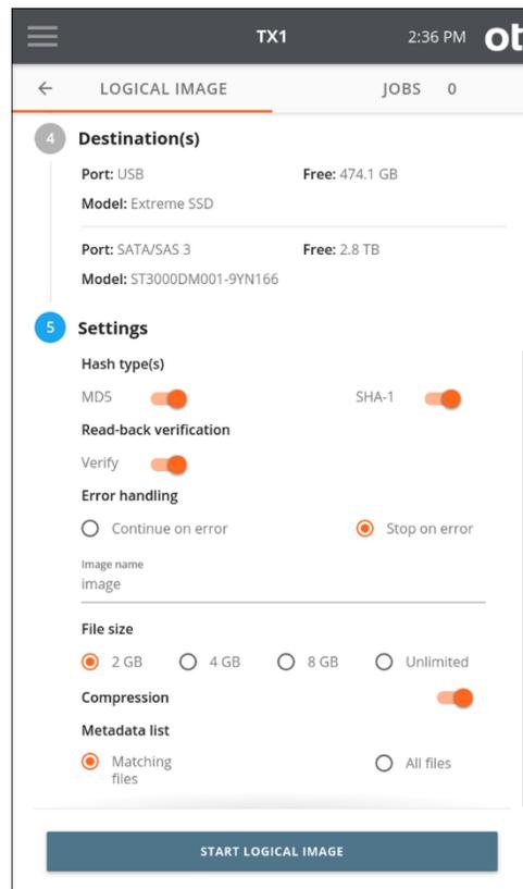
Select the desired **Hash type** for the logical image job - **MD5** and/or **SHA-1**. Note that hash values for source files will be calculated based on the chosen hash settings, even if no **lx01** outputs are requested. In that case, the file data is still read to allow for hash calculation, and the file-based hash values are stored in the metadata output file.
