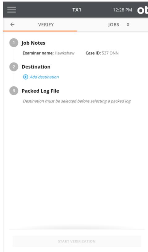
3. Select a **Packed log file**. Browse the destination and locate an existing TX1 packed log file.
