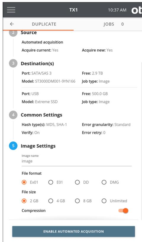
**Image name** defines the base filename for image segments. The default value is image. Tap the **Image name** text area to change the filename, then select a **File format** and **File size**.
