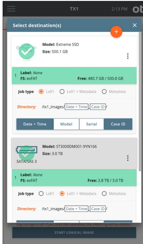
Destination drives with no recognized filesystems are grayed out, with a warning message stating no filesystem is available. Such a drive can be formatted through the media utilities available on the drive details screen, which can be accessed by tapping the additional options menu (three vertical dots) at the right side of the drive tile, or from the **Destinations** button on the **Home** screen.
