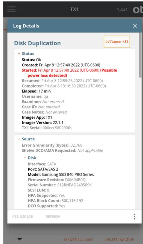
TX1 also allows the resumption of imaging jobs that failed for the following reasons:
