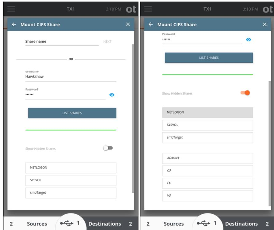
5. Enter a nickname for this CIFS share (optional) and enter a login username and password (if required). Choose the **SMB Version** and enable SMB 3.0 encryption (if desired), then tap the **Mount** button to login and mount the CIFS share.
